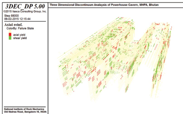
Fig. 11 - State of rock bolts in the caverns
